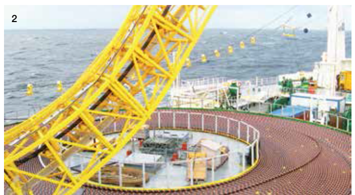
1 Typical cable laying and trenching operation | 2 Coiled cable on small cable laying barge.
